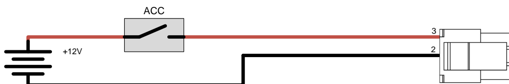
Figure 10: Remote enable configuration example – vehicle key switch
