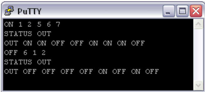
Figure 7: An example using PuTTY to control the PowerHub.
